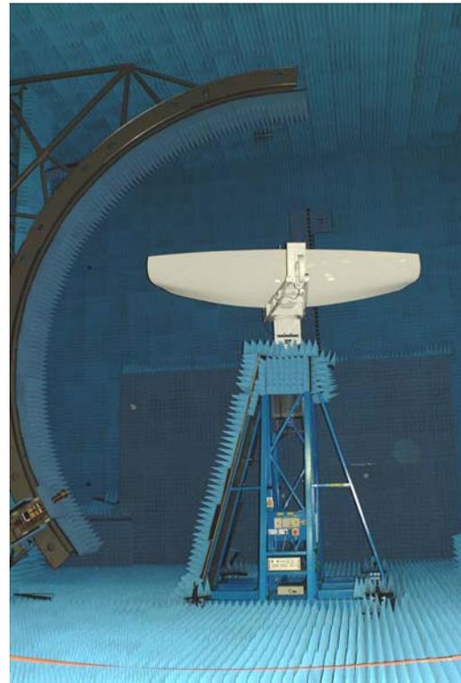
**Figure 1 Photo of Arch, AUT and Mounting Structure**
