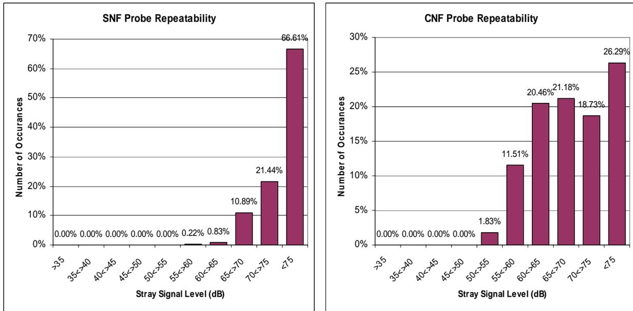
**Figure 4: (a) SNF and (b) CNF Probe Repeatability.** Histogram of the Equivalent Extraneous stray signals between two NF measurements with the probe moved 30mm between scans. Figure 4(a) corresponds to the patterns shown in Figure 3. The sample size for both figures was 1800 data points equally spaced from 0 to 360 degrees.
