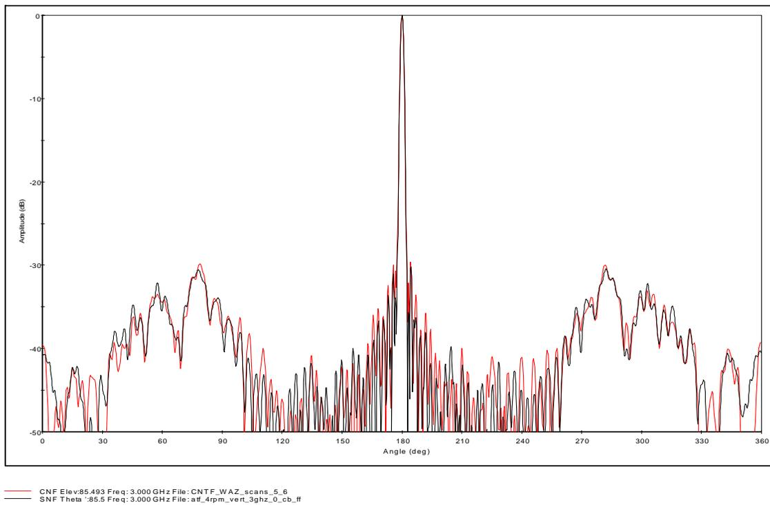
**Figure 5: CNF vs. SNF Azimuth Pattern Comparison**
