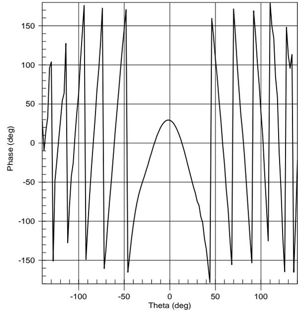
**Figure 1 Measured near-field phase for pyramidal horn antenna at 9.5 GHz.**
