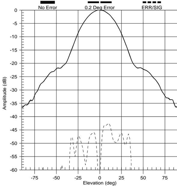
**Figure 3 Error signal level in the far-field pattern due to periodic theta position error of 0.2 degree.**
