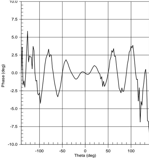
**Figure 2 Phase error for pyramidal horn antenna due to periodic theta position error of 0.2 deg.**
