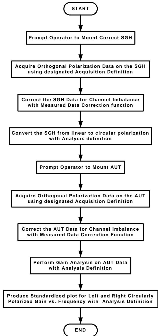
**Figure 1 -- Flowchart for Circular Gain Visual Basic Script**
