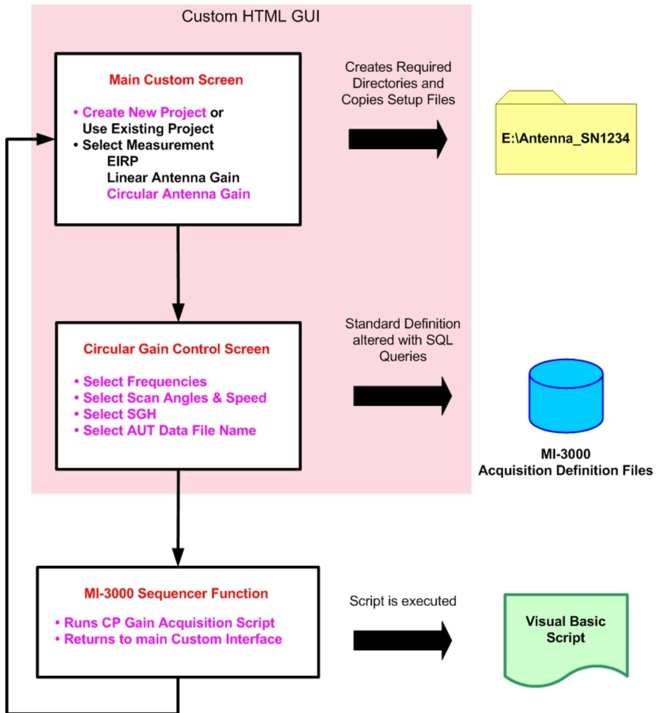
Figure 2 – Custom GUI Flowchart and Operations
