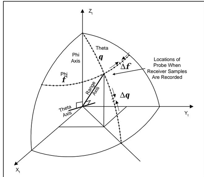
**Figure 1. The Measurement Coordinate System and Grid Points Representing Positions of the Probe Origin when the Received Signal is Sampled.**
