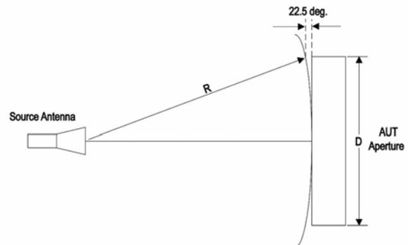
**Figure 1 - Far-field Distance Determination**
