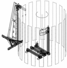
**Figure 7 - Cylindrical Near-field Range**
