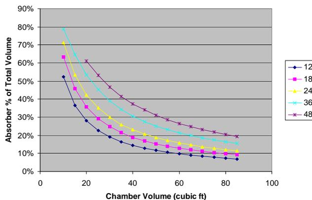
**Figure 10 - Chamber Absorber Volume**
