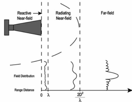
**Figure 5 - Fields of a Radiating Antenna**
