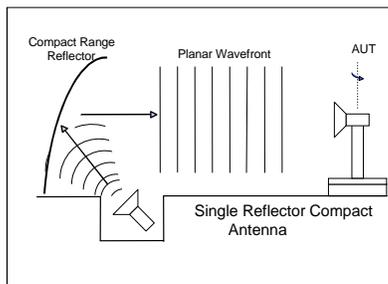
**Figure 4- Single Reflector Compact Range**
