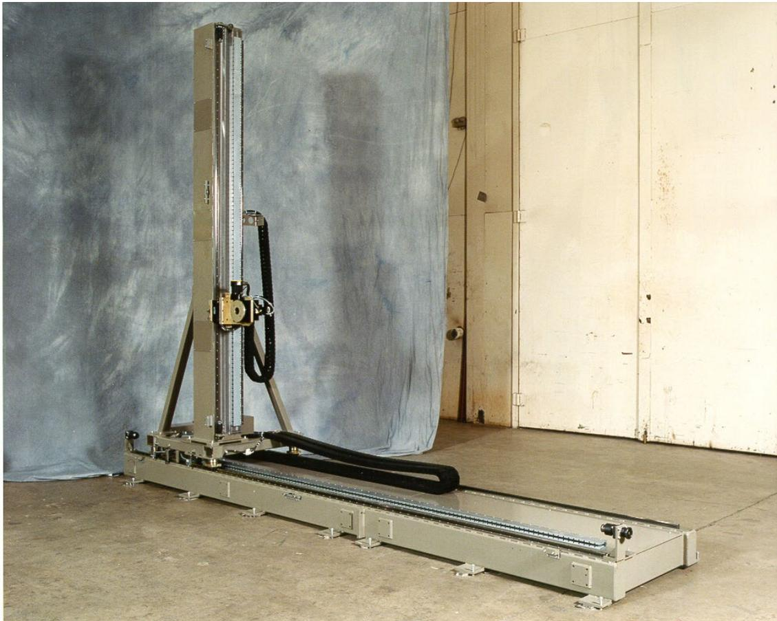
**Figure 3. A Typical Planar Near-Field Scanner.**
