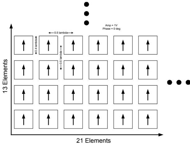
**Figure 2: Enlarged section of Figure 1 showing array element size and spacing.**
