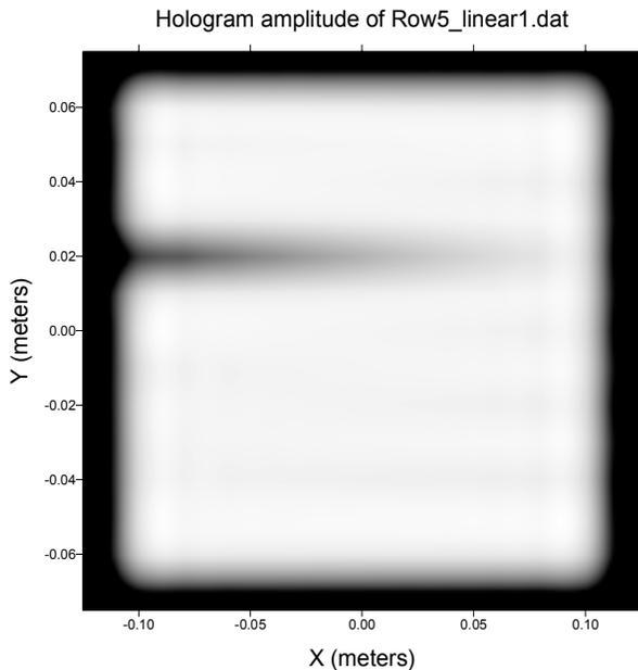
**Figure 11: Field amplitude of the back projected data for the array shown in Figure 1 with a linear attenuation factor introduced for the excitation of row 5.**
