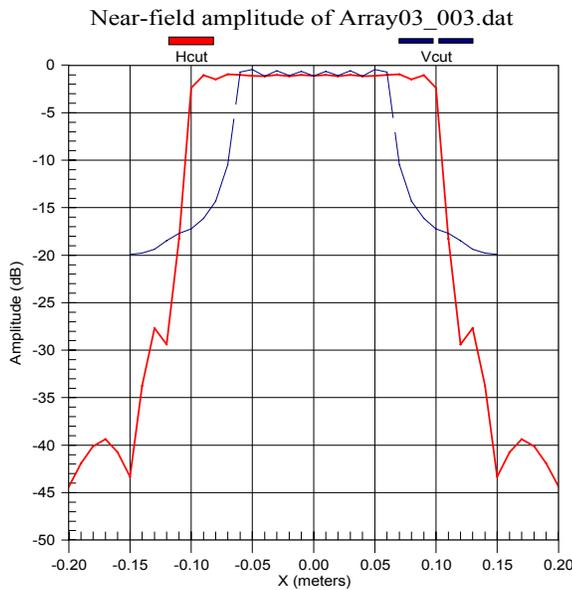
**Figure 3: Orthogonal near-field pattern cuts close to the surface of the array.**
