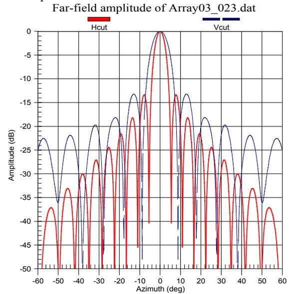
**Figure 4: Principal plane pattern cuts for the uniform array distribution shown in Figures 1 & 2.**
