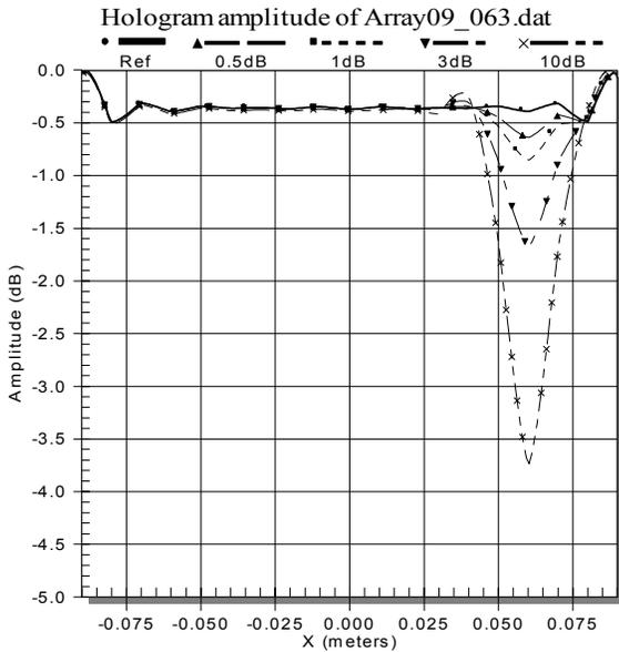
**Figure 9: Amplitude change in the back projected field for excitation amplitude change of a single array element.**
