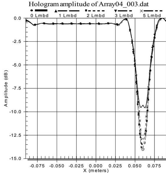
**Figure 7: Amplitude of the back projected data for different probe to AUT separation distances.**
