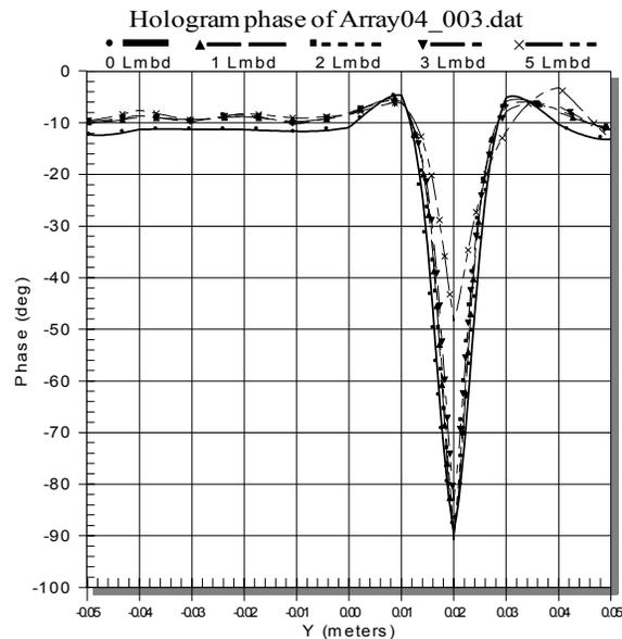
**Figure 8: Phase of the back projected data for different probe to AUT separation distances.**
