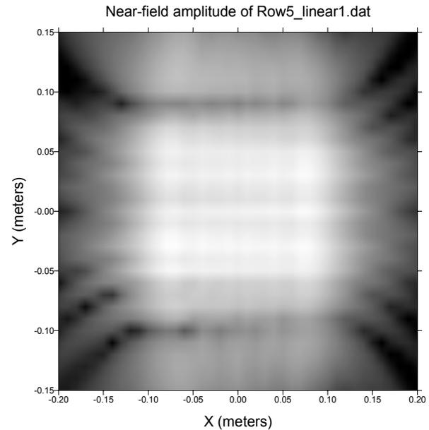
**Figure 10: Raw near-field amplitude ( $3\lambda$ ) for the array shown in Figure 1 with a linear attenuation factor introduced for the excitation of row 5.**
