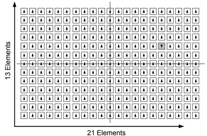
**Figure 5: The location is shown of the single element with reversed phase.**
