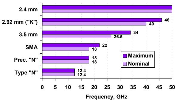
Figure 4 Commonly Used Coaxial Connectors
