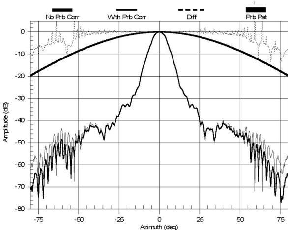
**Figure 9: The impact of OEWG probe correction on the co-polar azimuth pattern cut.**
