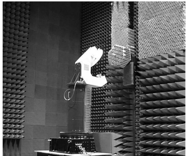
**Figure 3: Cylindrical near-field measurement test configuration.**
