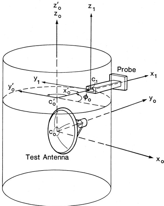
**Figure 2: Cylindrical near-field coordinate system.**
