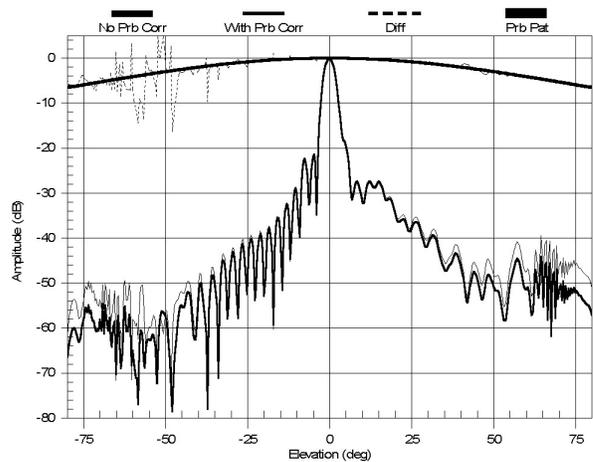
**Figure 10: The impact of OEWG probe correction on the co-polar elevation pattern cut.**
