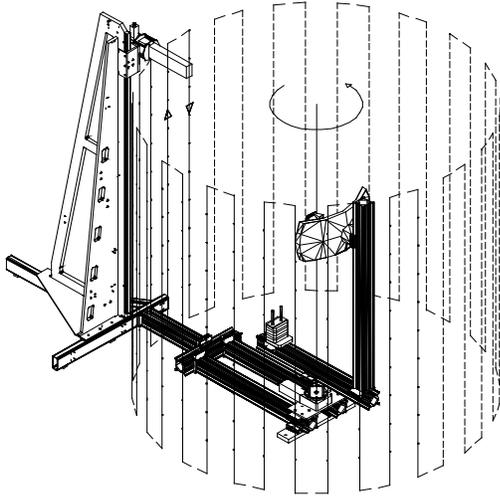
**Figure 1: Typical cylindrical near-field data acquisition system.**
