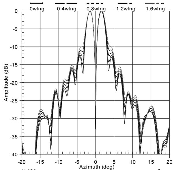
Figure 7: Azimuth difference patterns for radial distance errors.
