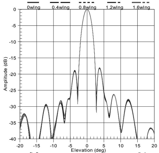
Figure 6: Elevation radiation pattern data for multiple cylindrical near-field data sets with radial distance parameter offset values introduced.
