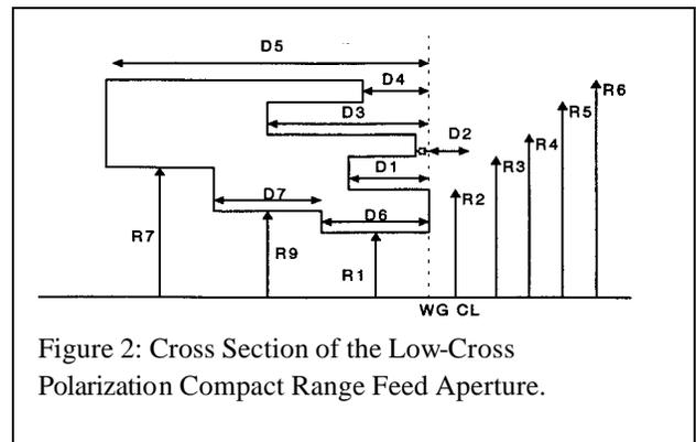
Figure 2: Cross Section of the Low-Cross Polarization Compact Range Feed Aperture.
