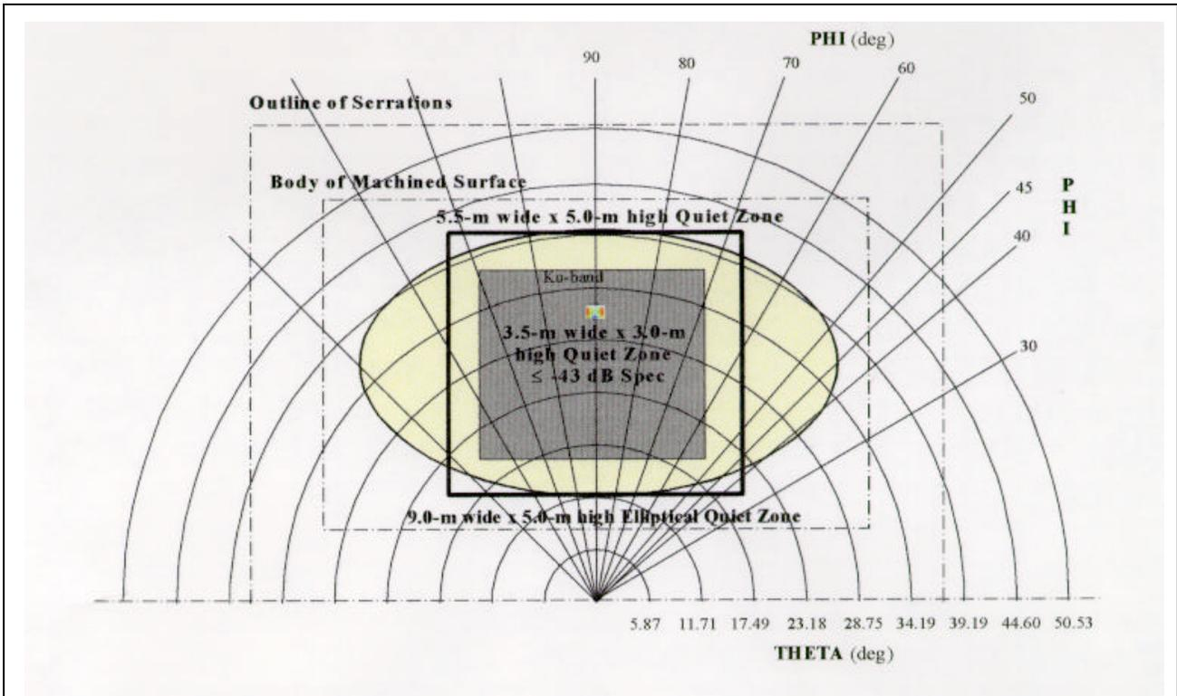
Figure 1: Compact Range Feed pointing angles overlaid on the Layout of the Quiet Zone of a MI Technologies Model 5712 Compact Antenna Range Reflector.
