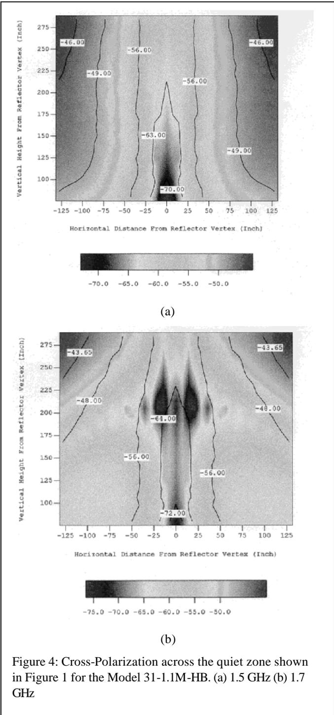
Figure 4: Cross-Polarization across the quiet zone shown in Figure 1 for the Model 31-1.1M-HB. (a) 1.5 GHz (b) 1.7 GHz
