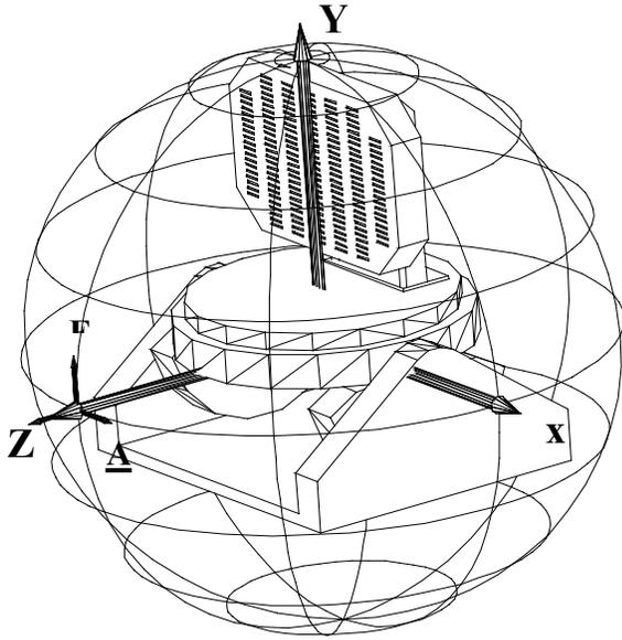
**Figure 2 Azimuth over elevation coordinate system and the associated vectors A and E.**
