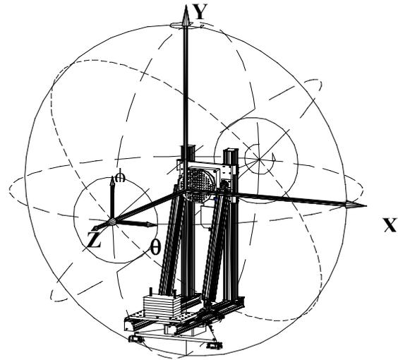
Figure 1 Theta Phi coordinate system and vector components
