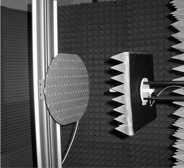
**Figure 4 Slotted array test antenna in its initial un-rotated orientation.**
