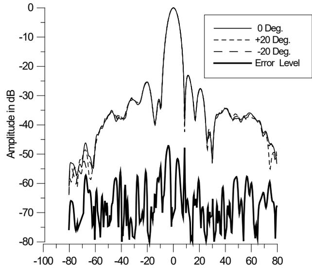
**Figure 8 Using comparison of rotated patterns to estimate error levels.**
