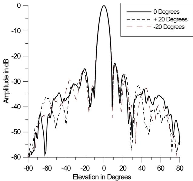
**Figure 7 V-cuts through beam peak for three azimuth rotations of the AUT. Alpha Epsilon coordinates and vector components used.**
