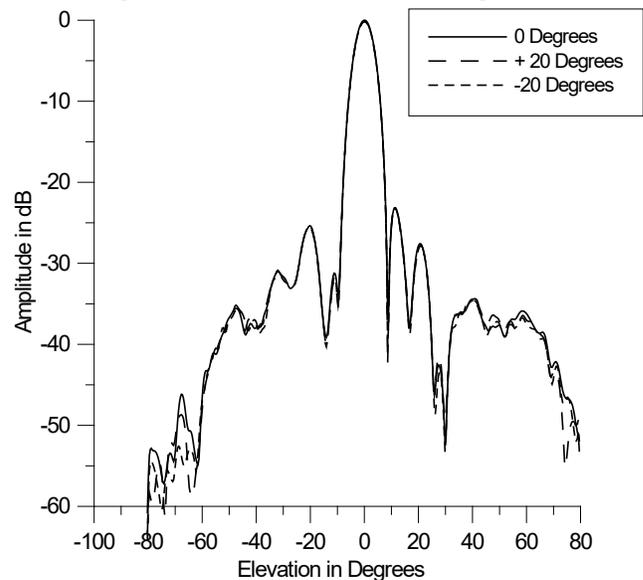
**Figure 6 V-cuts through beam peak for three azimuth rotations of the antenna. Az EL coordinates and vector components used.**
