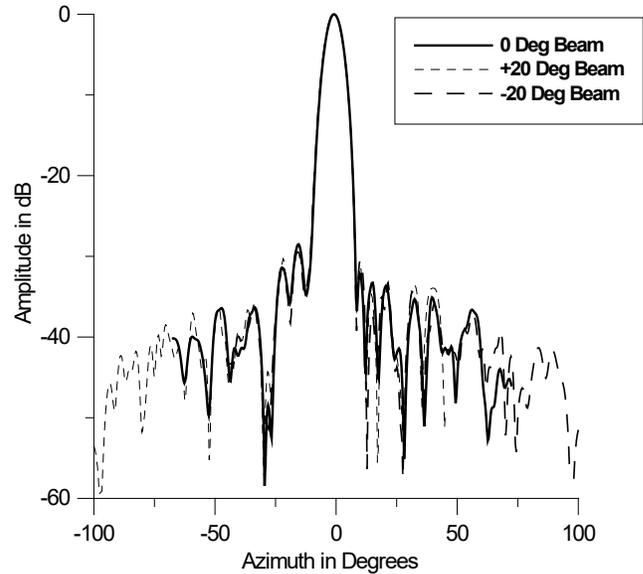
**Figure 5 Angular coverage increased by combining steered beams.**
