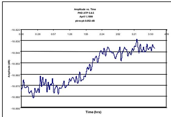
**Figure 9 RF Thermal Stability - Amplitude**
