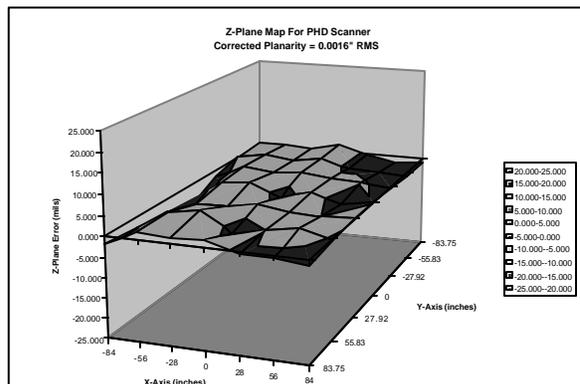
**Figure 8 Z-Planarity (corrected)**
