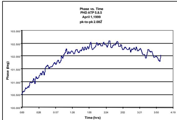
**Figure 10 RF Thermal Stability - Phase**
