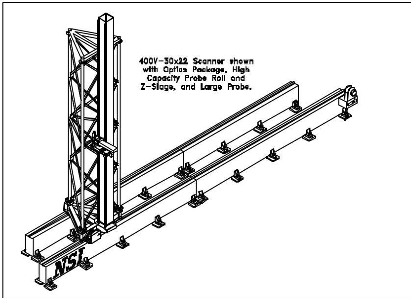
*Figure 3 A drawing of the 9m x 6.4m planar scanner.*
