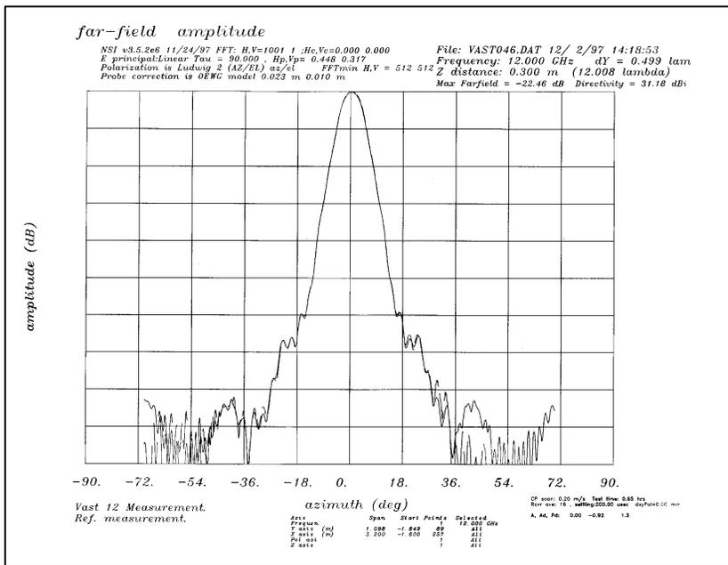
**Figure 6** Far-field azimuth reference pattern and pattern for the AUT #2 offset by -20 degrees in azimuth are shown superimposed as part of the system validation testing. (The offset pattern is shown shifted back to 0 here for comparison purposes.)
