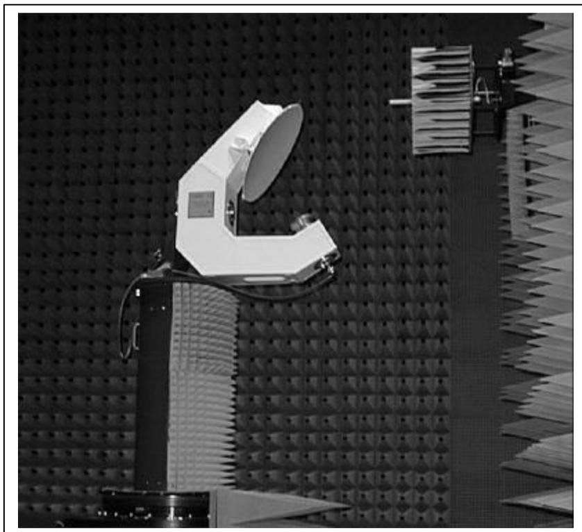
*Figure 4 The ESA/ESTEC Vast12 antenna (used for chamber validation) is shown mounted in the chamber. Note the high power probe absorber.*
