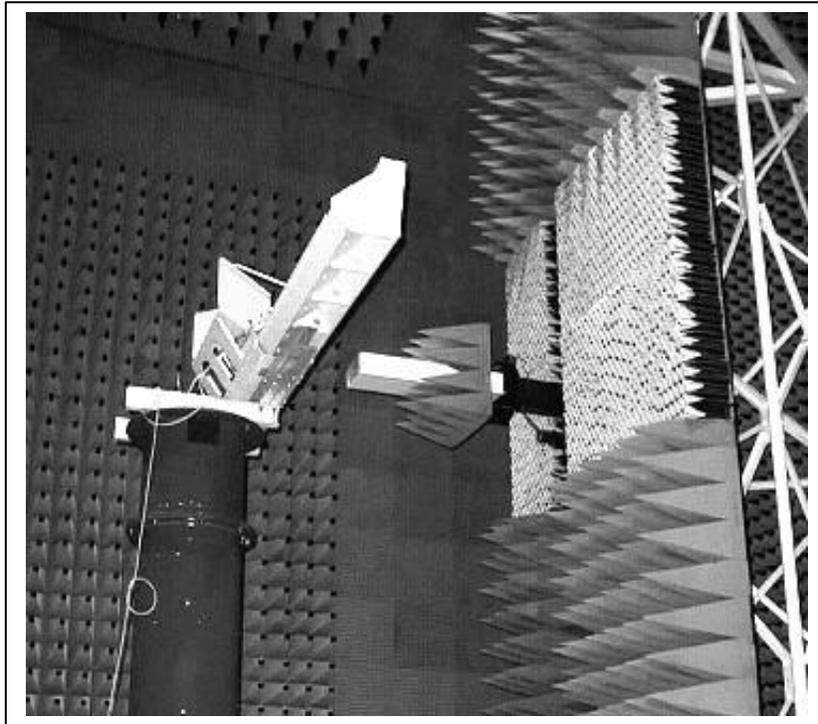
**Figure 5** The linear array (Antenna #3) shown mounted in the RNN chamber.
