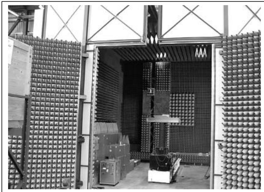
*Figure 2 The chamber slotted ceiling allowing crane access is shown.*
