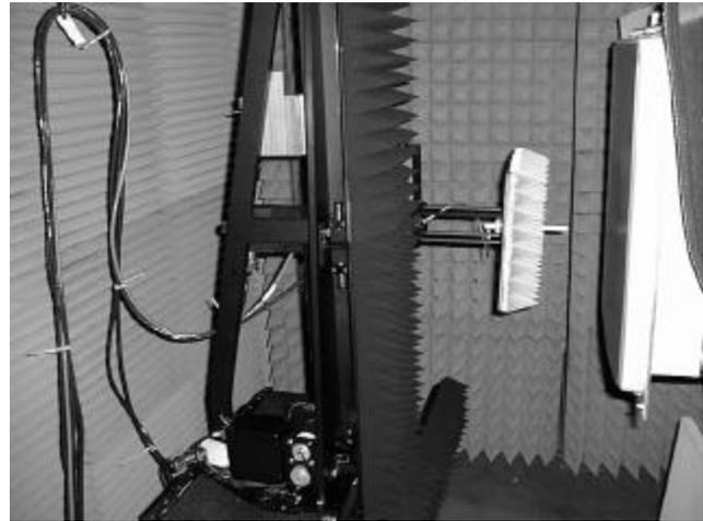
Figure 3 DVS antenna and nearfield scanner
