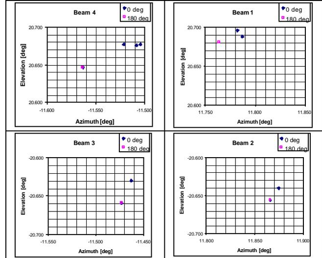
Figure 5 Boresight results for all 2-way beams
