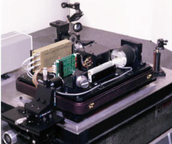
*Figure 4 NSI Laser Optical Position Measurement System*
