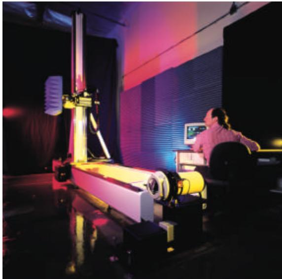
Figure 1 TNAMS 12' x 9' Near-field Scanner
