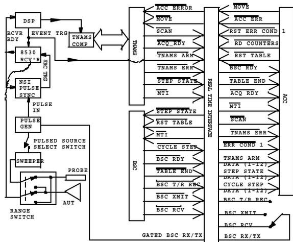
Figure 5 AAMTB Signal Control Diagram
