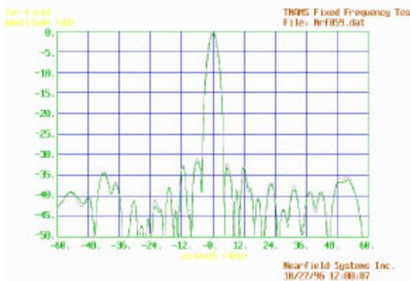
Figure 8 Antenna Pattern Overlay (CW & Pulse)
