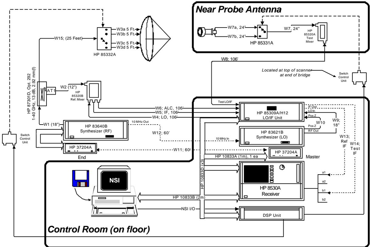
Figure 5. Lockheed RF System Block Diagram – Transmit from AUT
