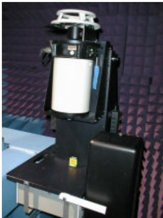
Figure 3 Spinning plane Z laser with XY laser below plate
