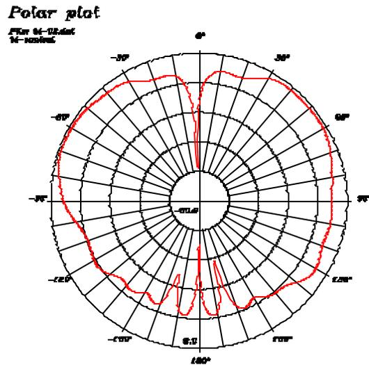
Figure 9 Broadbeam Bi-Conical Antenna Pattern
