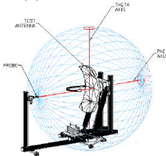
Figure 1 Spherical Measurement System
