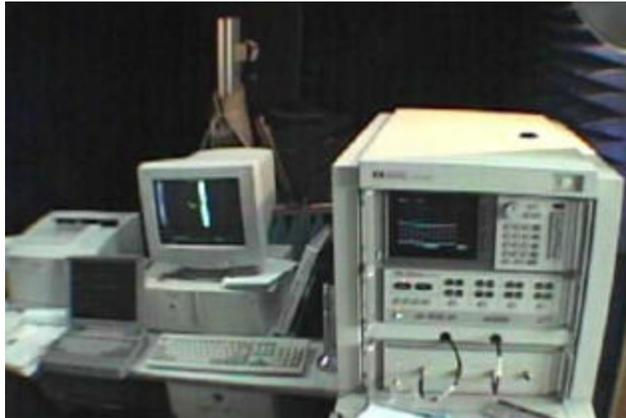
Figure 2 HP 85301C Network Analyzer
