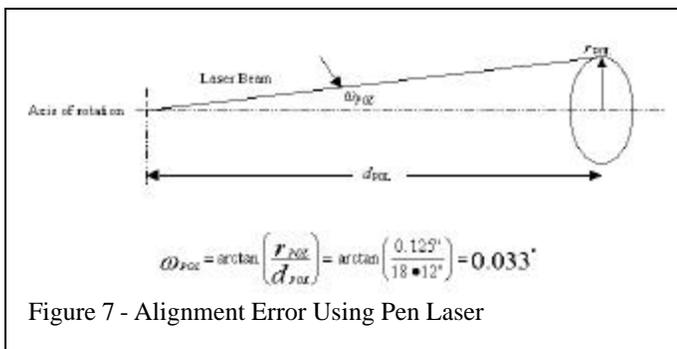
Figure 7 - Alignment Error Using Pen Laser
