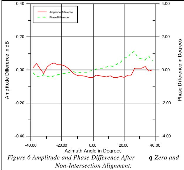
Additional adjustments could be made to improve the alignment, but from Fig. 6 it is apparent that the  $\theta$ -zero error is less than 0.04 deg. and the non-intersection is less than 0.01 cm which is adequate for this antenna/frequency.
