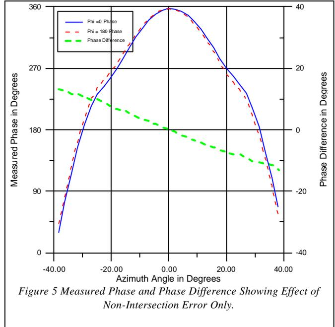
Figure 5 Measured Phase and Phase Difference Showing Effect of Non-Intersection Error Only.
