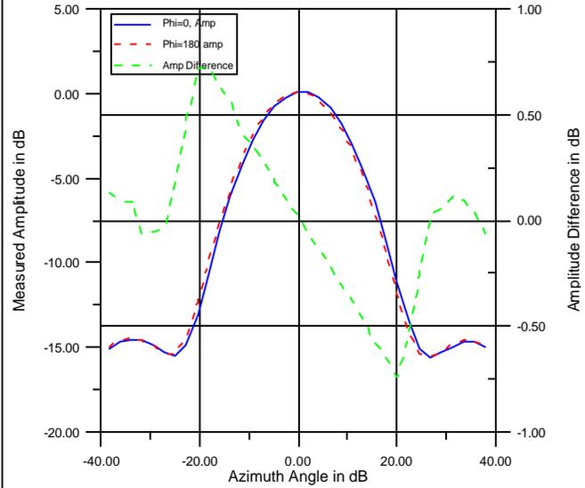
Figure 3 Measured Amplitude and Amplitude Difference Showing Effect of  $q$ -zero and  $X$ -zero Alignment Errors.
