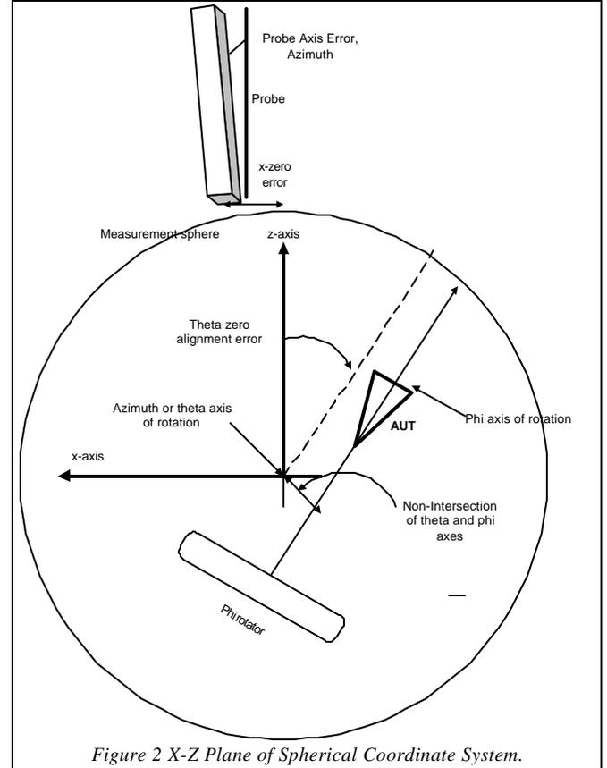
Figure 2 X-Z Plane of Spherical Coordinate System.
