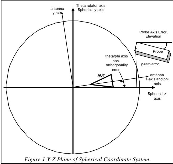
Figure 1 Y-Z Plane of Spherical Coordinate System.
