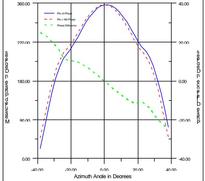
Figure 4 Measured Phase and Phase Difference Showing Effect of  $q$ -Zero and  $X$ -Zero and Non-Intersection Alignment Errors.
