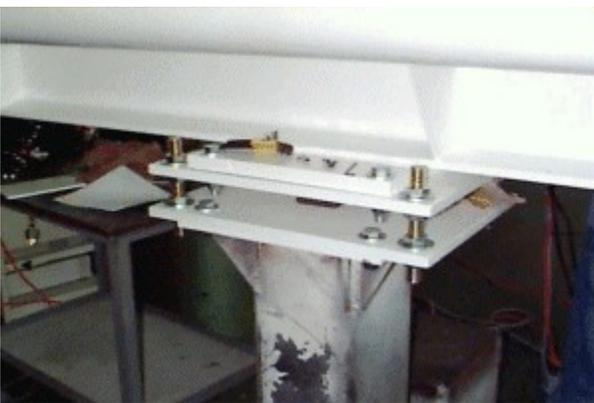
**Figure 10. Scanner Foot Mounting Pad**
