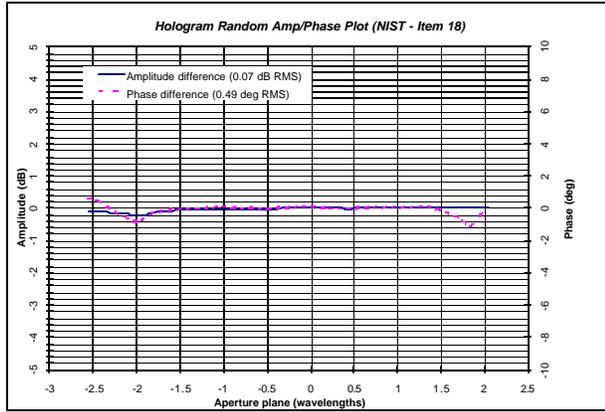
Figure 4 Random Amplitude and Phase Error Plot
