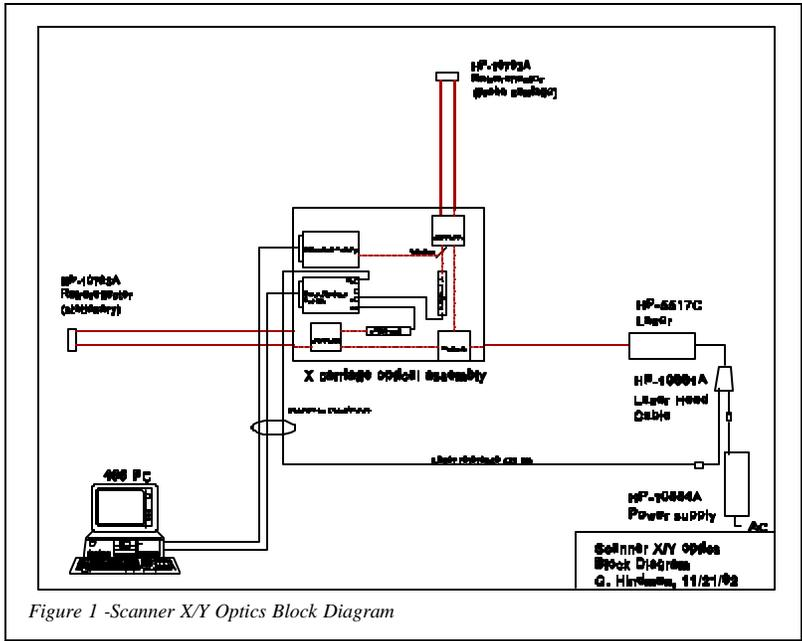
Figure 1 -Scanner XY Optics Block Diagram
