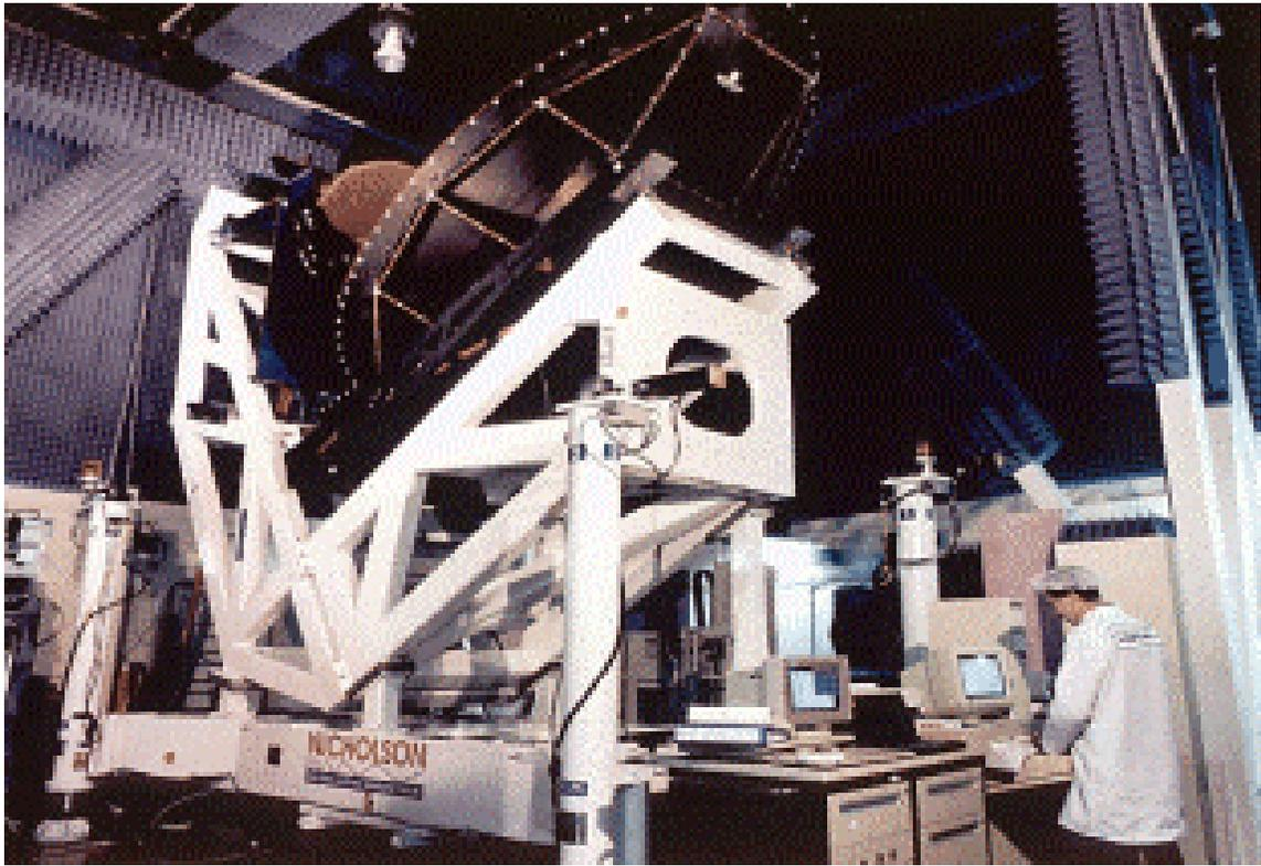
*Figure 3 - NSI Scanner Testing SS/L Antenna*
