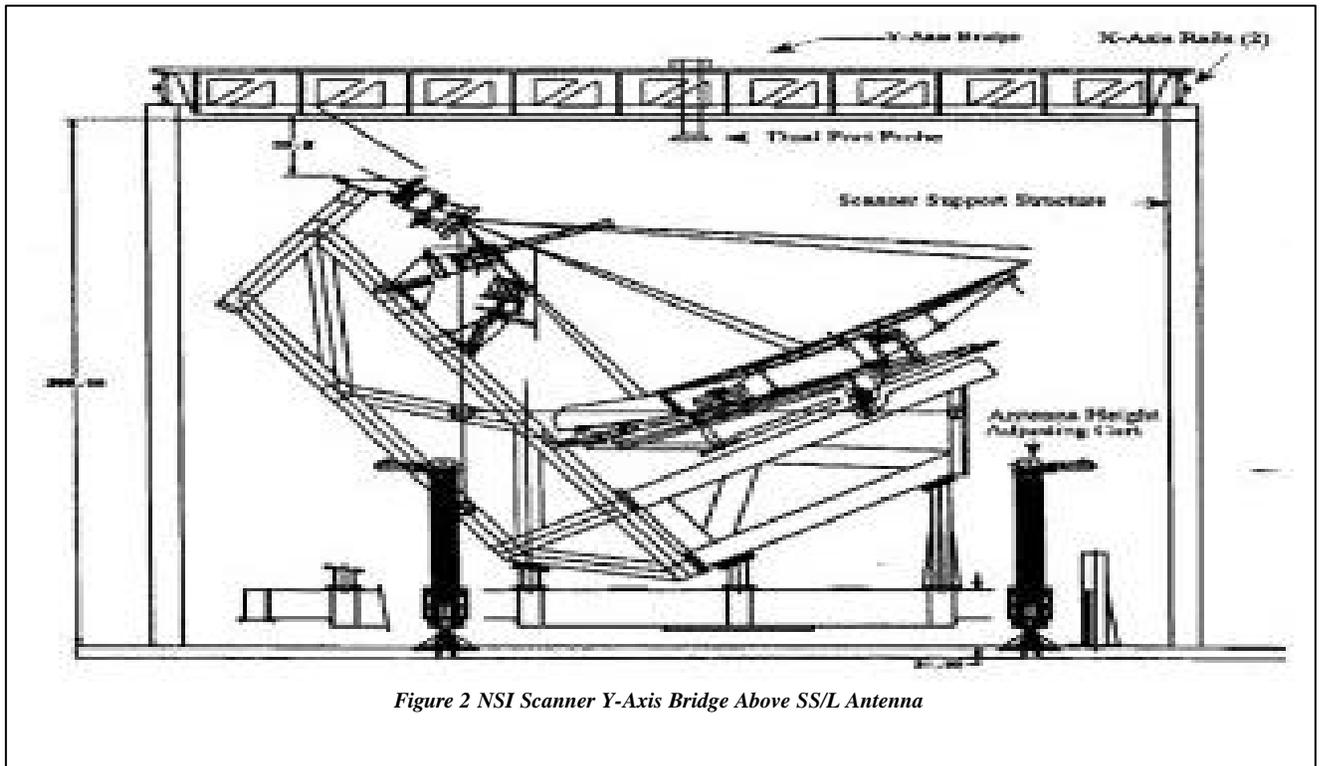
Figure 2 NSI Scanner Y-Axis Bridge Above SS/L Antenna
