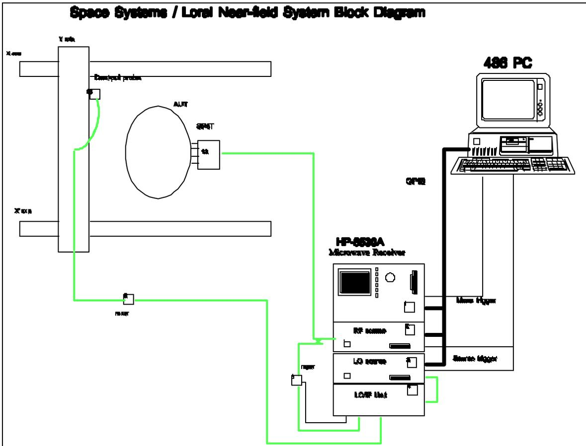
Figure 5 - SS/L RF Sub-system Block Diagram
