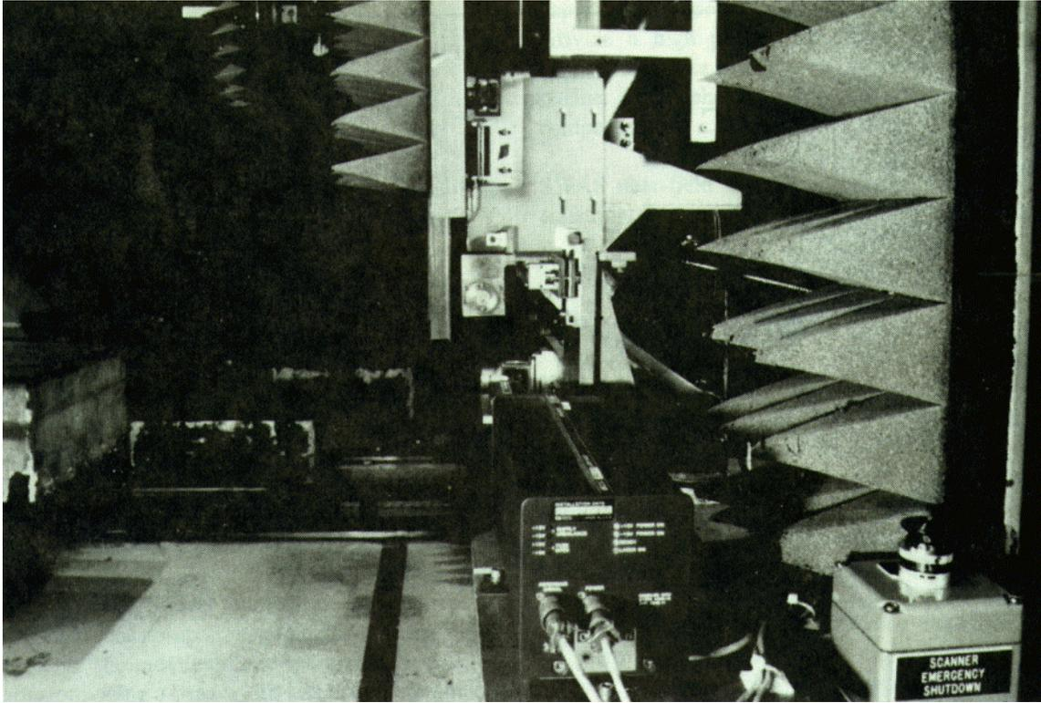
Figure 2 Hughes Space & Comm Nearfield Scanner Laser Interferometer
