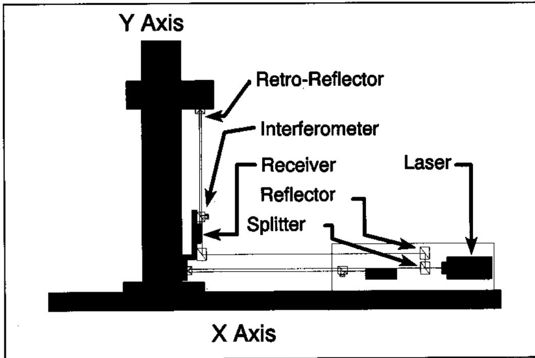
Figure 3 Hughes Scanner Laser Optics
