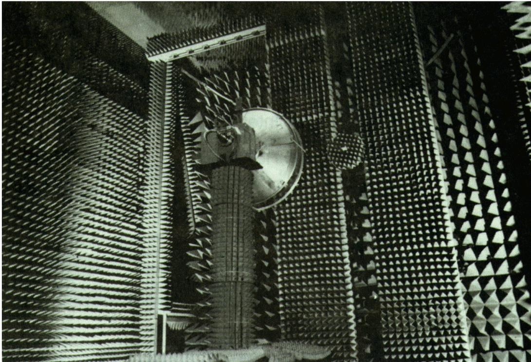
*Figure 1 Hughes Space & Comm 12' x 12' Vertical Nearfield Scanner*
