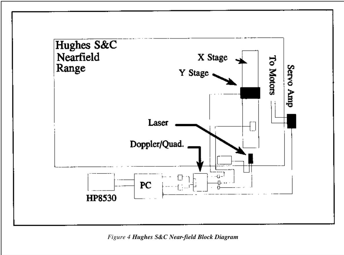
Figure 4 Hughes S&C Near-field Block Diagram
