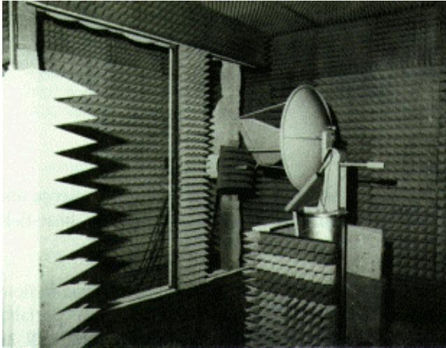
*Figure 1 NSI 5' By 5' Planar/Cylindrical Near-Field System*
