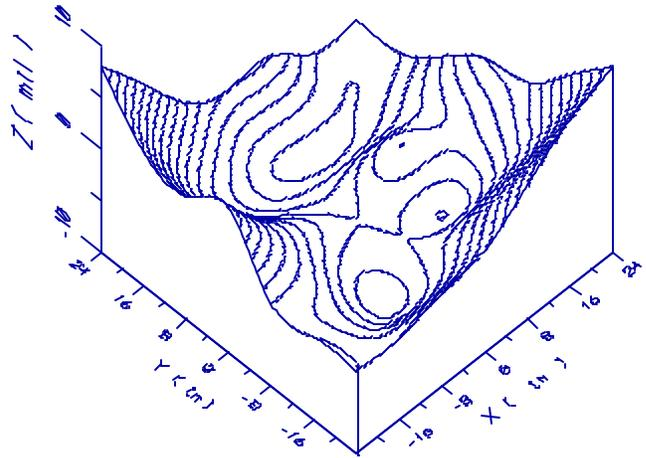
Figure 6 Scanner Z-plane errors
