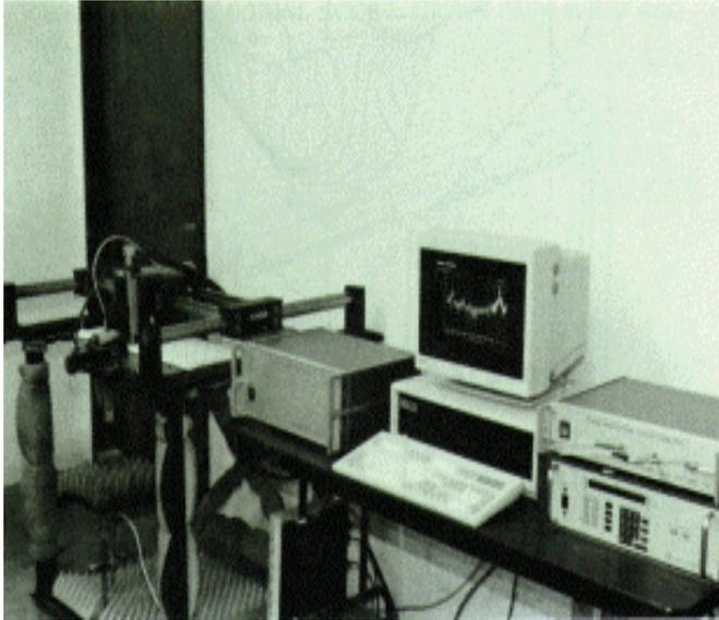
Figure 7 *Portable System And Phase Modulated Interferometer*
