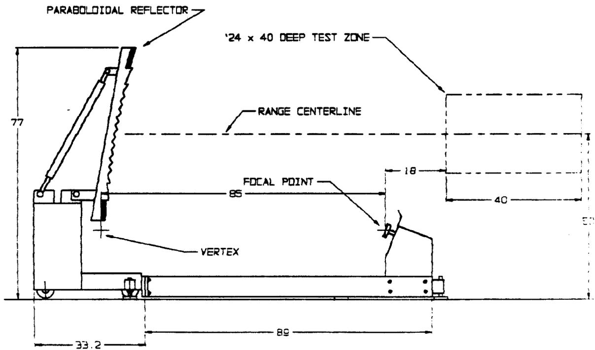
Figure 2. Model 5702 Virtual Vertex Compact Range
