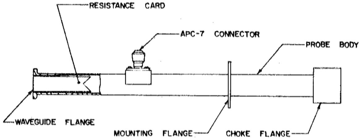
**Figure 2 Dual-Polarized Spherical Near-Field Probe**
