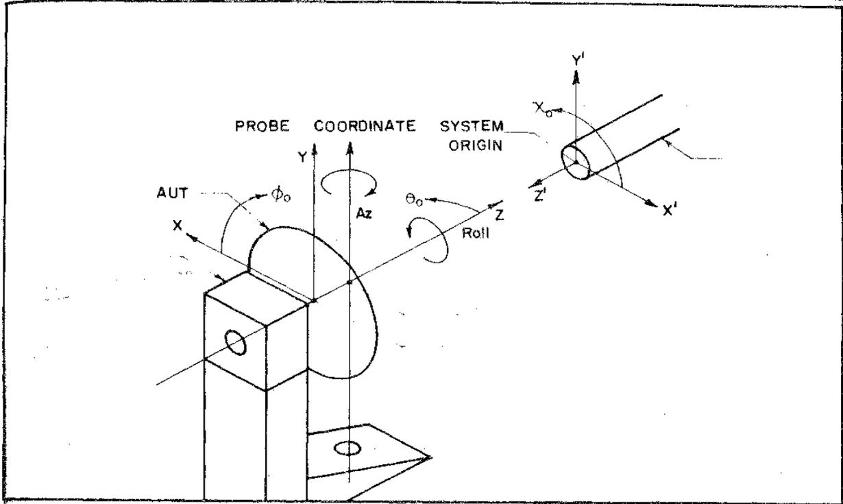
**Figure 1 Coordinate System for Spherical Near-Field Scanning**
