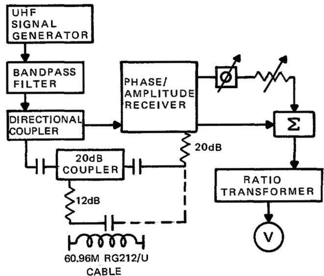
Fig. 5. Cable and coupling network loss measurement.
