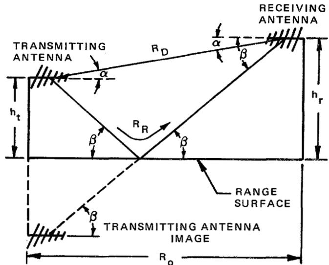
Fig. 1. Range configuration for calibrating gain of wide-beam antenna.
