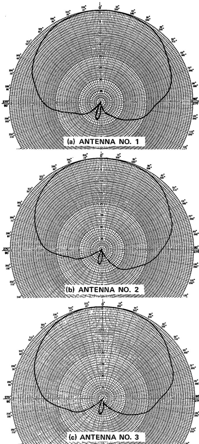
Fig. 4. H plane pattern of three UHF gain standards at 300 MHz (dB scale).
