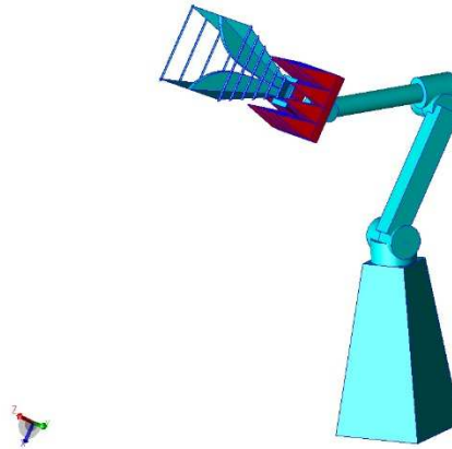
Figure 1: A dual ridged antenna is used as a broadband probe with an industrial robotic arm. The model is rotated to study the effect of the arm on the probe illumination at different arm positions.
