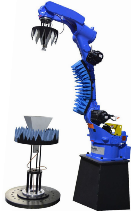
Figure 1: Robotic scanner used for spherical near-field measurements
