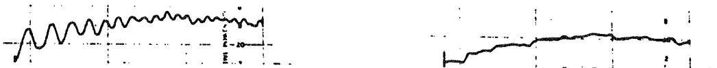
Fig 2. A comparison of data at 10 GHz showing the effect on the horizontal amplitude traces created by masking the left serrated edge with a line of absorber panels. The probe antenna used was a 30^\circ beamwidth diagonal horn. The length of travel is 6.5 ft.
