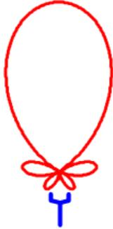
Fig. 1 Schematic of a Bare Antenna and Its Radiation Polar Diagram
