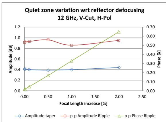
Fig. 14. Simulated variation of quiet zone performance with progressive defocusing of the CATR reflector, vertical cut, horizontal polarization
