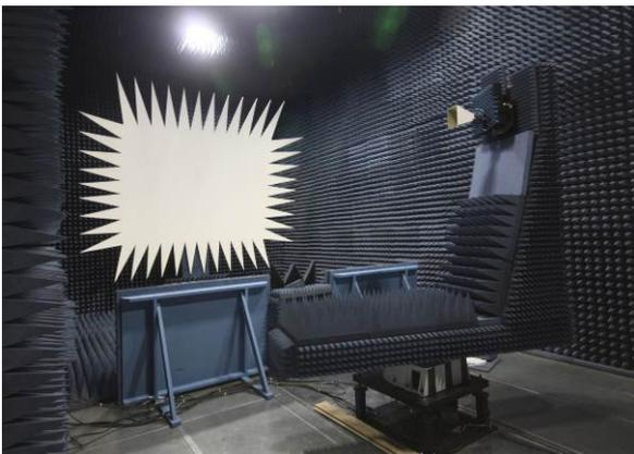
Fig. 2. CATR portion of range; the AUT positioner is shared with the SNF system
