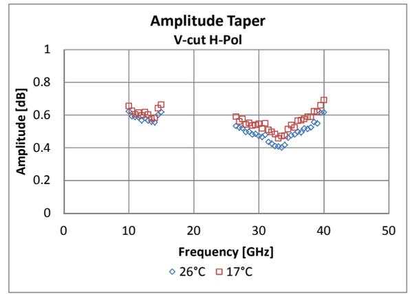
Fig. 11. QZ amplitude taper comparison at 26°C and 17°C
