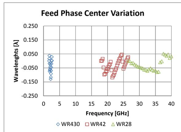
Fig. 4. Variation of phase center with frequency
