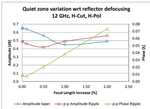
Fig. 15. Simulated variation of quiet zone performance with progressive defocusing of the CATR reflector, horizontal cut, horizontal polarization
