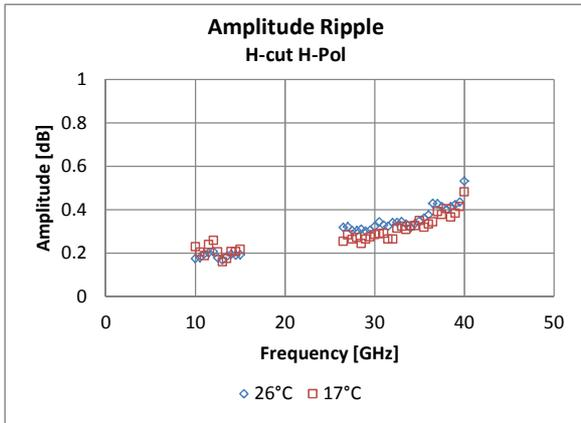
Fig. 9. QZ amplitude ripple comparison at 26°C and 17°C
