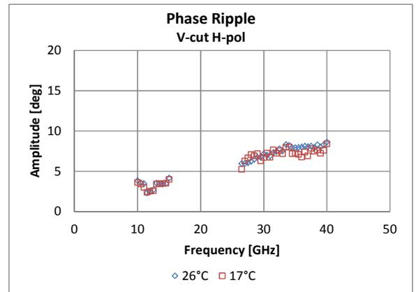
Fig. 13. QZ phase ripple comparison at 26°C and 17°C
