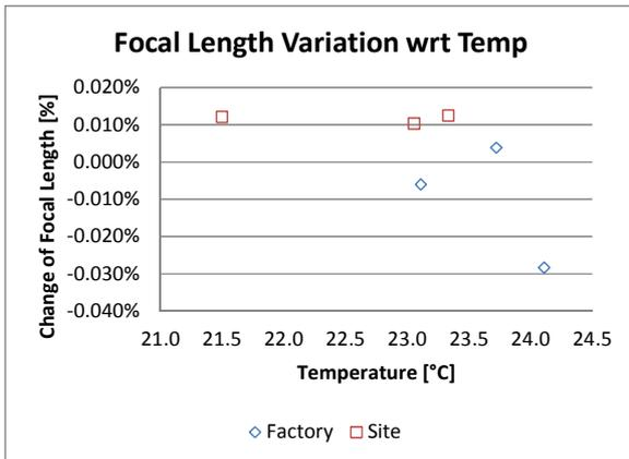
Fig. 5. Variation of reflector focal length with respect to temperature
