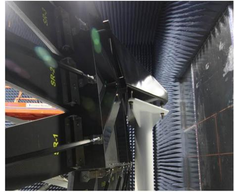
Fig. 3. Rear of carbon-fiber CATR reflector; the carbon-fiber support mount can be seen on the pedestal
