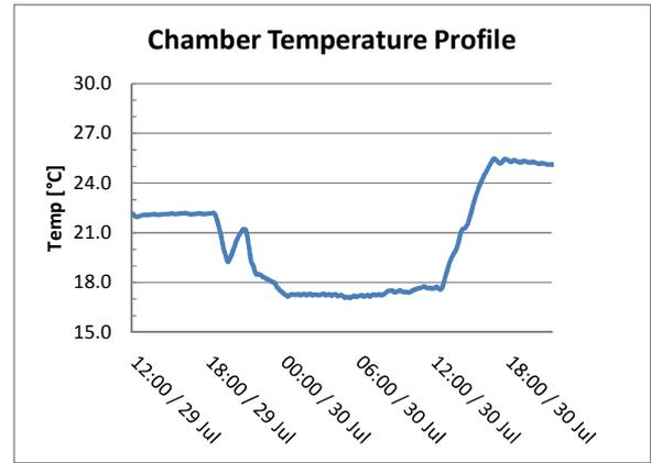
Fig. 6. Chamber temperature was cycled from 17 – 26°C allowing for the chamber to achieve thermal equilibrium in both temperature extremes
