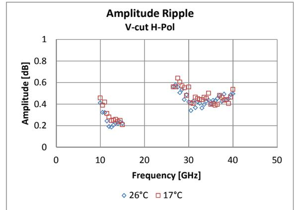
Fig. 12. QZ amplitude ripple comparison at 26°C and 17°C
