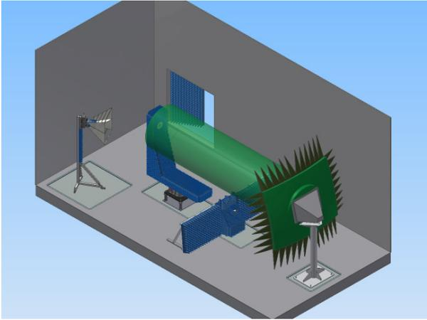
Fig. 1. Mechanical drawing of the combination CATR / SNF range
