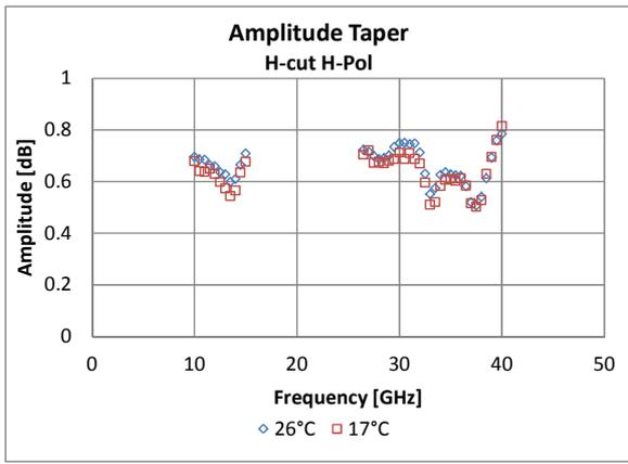
Fig. 8. QZ amplitude taper comparison at 26°C and 17°C
