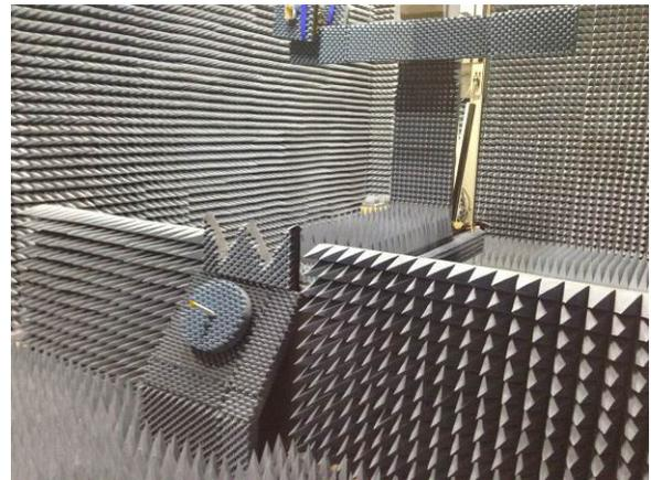
Fig. 7. Test setup with the field probe can be seen in horizontal orientation and mounted on the AUT positioner
