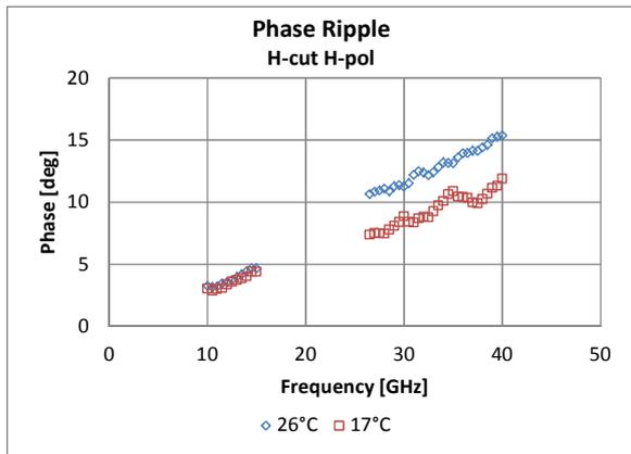
Fig. 10. QZ phase ripple comparison at 26°C and 17°C
