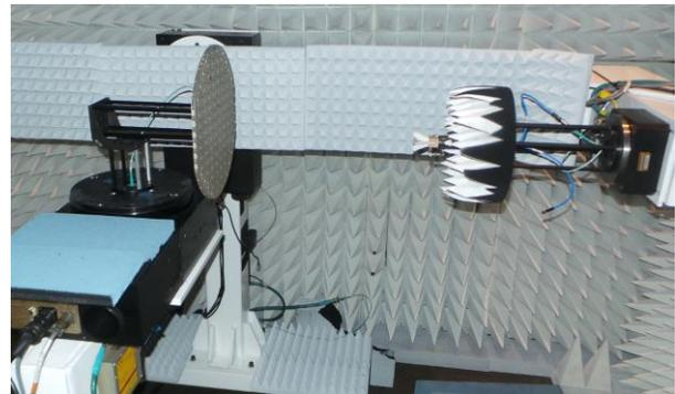
Figure 5. SWGA Mounted in Equatorial Mode with NSI Dual-Polarized Probe Mounted to Theta Swing Arm. (Phi=0° and Theta=90° Shown Here)
