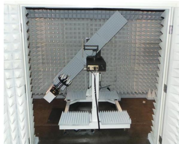
Figure 4. X-Band Slotted Waveguide Array Under Test on the NSI-700S-110 SNF System
