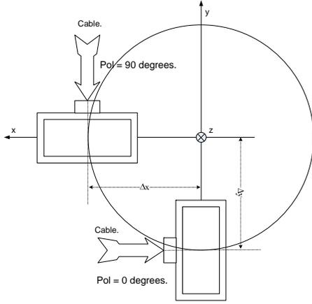
**Figure 1: Schematic of spherical measurement system showing probe axis alignment error. Here probe translation from  $\chi = 0^\circ$  position to  $\chi = 90^\circ$  position is shown.**
