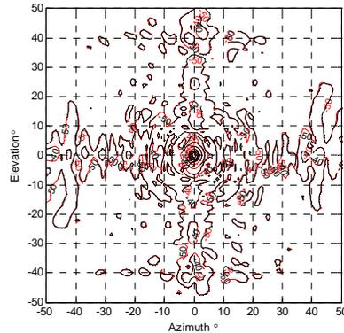
**Figure 16 Red denotes reference far-field pattern, black denotes  $0.1\lambda$   $x$ -axis offset probe at a measurement radius of  $4\times\text{MRE}$ .**
