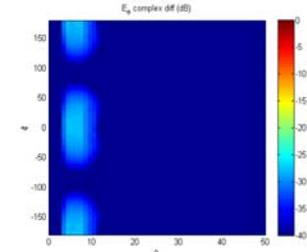
**Figure 13: Difference amplitude peak = -27.5 dB near-field pattern for  $\Delta x=0.1\lambda$  and measurement radius =  $4\times\text{MRE}$ .**
