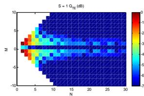
**Figure 6: False colour plot of SMCs of first order probe offset by  $0.2\lambda$  in  $x$ -axis**
