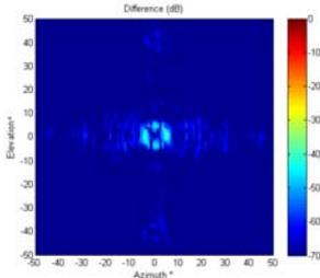
**Figure 16: amplitude difference far-field pattern for  $\Delta x = 0.1\lambda$  and measurement radius =  $4\times\text{MRE}$ .**
