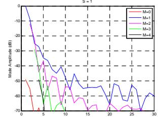
**Figure 5: Plot of SMCs of first order probe offset by  $0.1\lambda$  in  $x$ -axis.**
