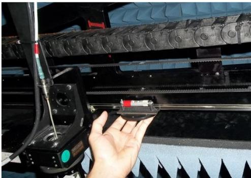
Figure 5. Checking the Radial Axis Level
