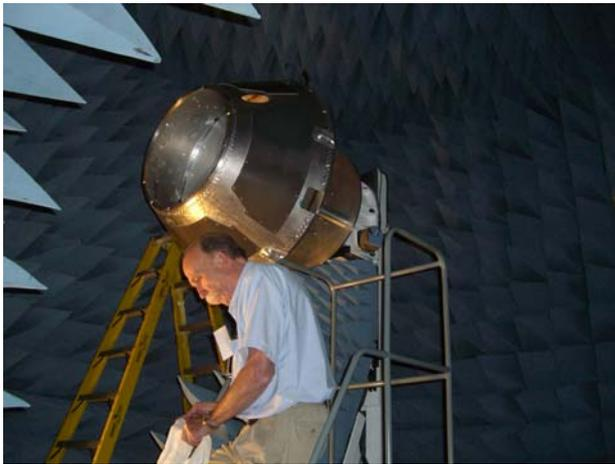
**Figure 7 – Mounting of the Flight Unit on the Phi Stage (Flight Unit Shown Before TPS Application)**
