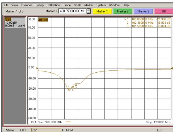
Figure 17 – Measured Return Loss of Flight Unit (Operational Frequency is Middle Marker)
