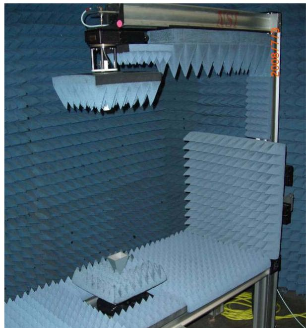
**Figure 5 – NSI-700S-80 Spherical near-field system testing X-band pyramidal horn.**
