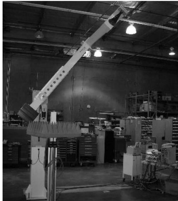
**Figure 6 OEWG probe on the arch spherical range without absorber enclosure.**
