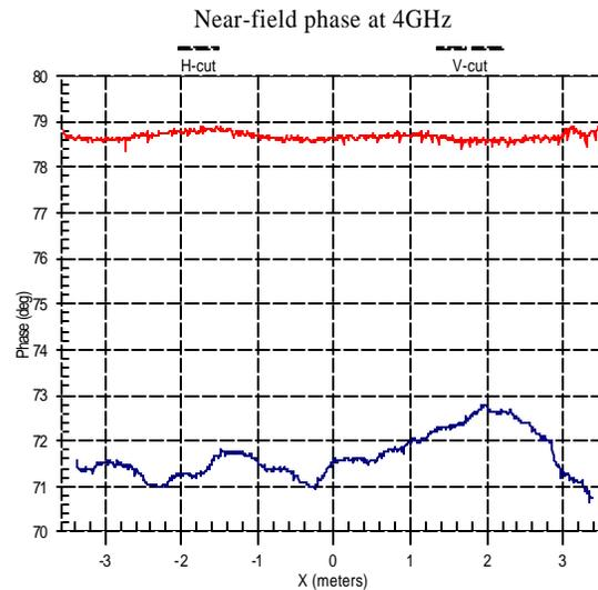
Figure 3: X-axis & Y-axis cable phase response at 4 GHz.
