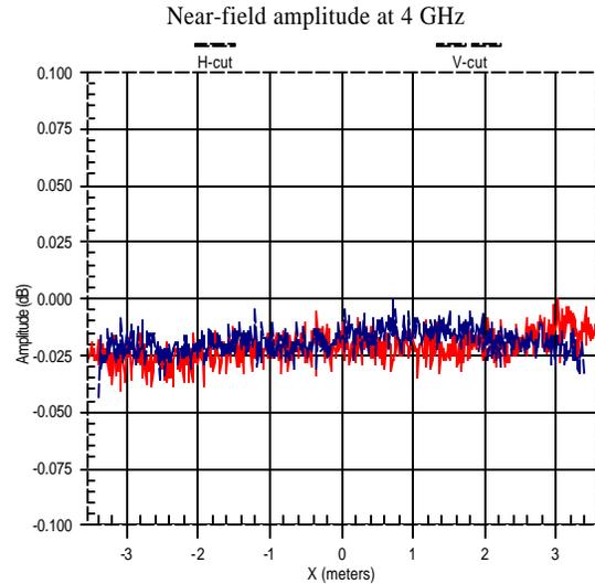
Figure 2: X-axis & Y-axis cable amplitude response at 4 GHz.
