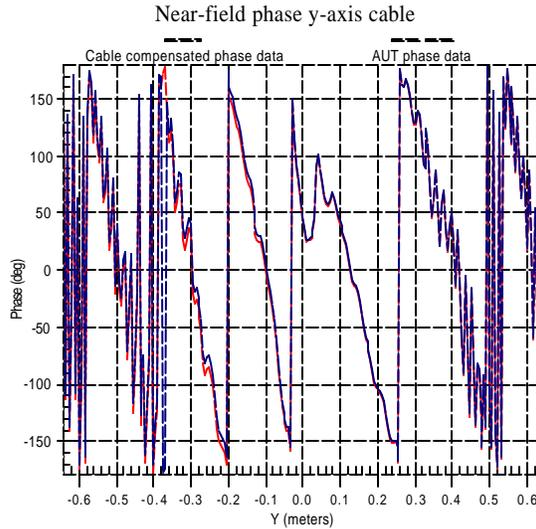
Figure 6: Measured near-field phase of AUT with and without cable effect.
