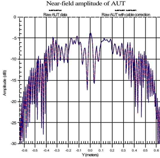
Figure 5: Measured near-field amplitude of AUT with and without cable effect.
