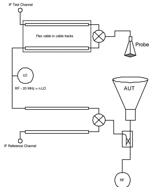
**Figure 1: Schematic diagram of the RF system and flex cables.**
