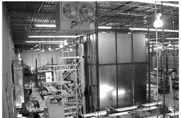
*Figure 3 Near-Field Test Chamber*
