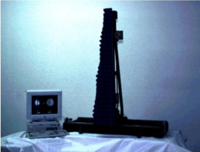
**Figure 1 - NSI Model 233L portable near-field scanning system.**
