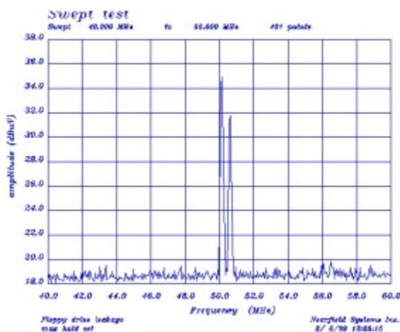
**Figure 2. Frequency plot showing maximum near-field electromagnetic interference levels near a floppy disk drive**
