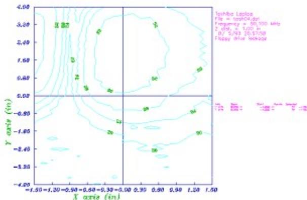
**Figure 3. This contour plot shows a spatial (XY) image of EMI emission near a floppy drive**
